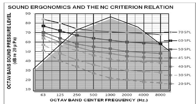
Fig. 6 Orchestra room sound pressure levels with the function of frequency. [9]
